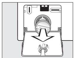
■ Remove the drain filter completely.
