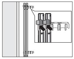
Secure the shipping struts to the back of the washing machine. Make sure that the top catch is located above the holder.
