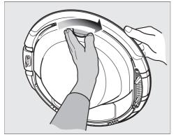
■ Turn the door in the direction of the arrow while pressing against the outer plate slightly with your flat hand.
