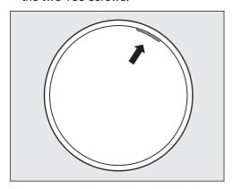
The yellow maker on the right-hand side shows operators and users which side to open the door.
