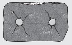
Lint will blow into the heat exchanger through cracks and tears. This will cause a permanent obstruction in the heat exchanger.
