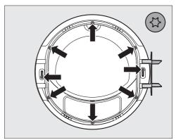
■ Use the Torx screwdriver to screw in the eight screws.
