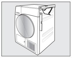
The appliance must stand perfectly level to ensure safe and proper operation.
