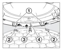
■ Looking in through the opening, position the door diagonally on the outer plate.
