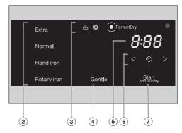
The ②, ④, ⑥, and ⑦ sensor buttons react to fingertip contact. Selection is possible as long as the respective sensor button is lit.
