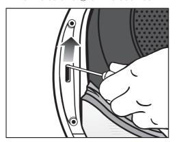
Use a screwdriver to push the door lock up.
