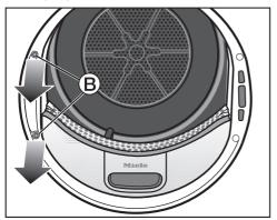
■ Use the Torx screwdriver to unscrew the two screws (B) on the door lock.
